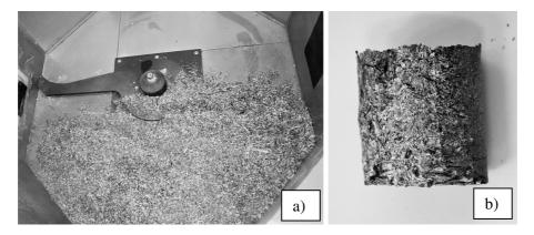
Fig. 2. Milled biomass material: a - bulk form - feedstock; b - densified form - briquette
