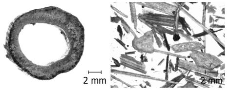
Fig. 3. Investigated feedstock material: a - cross-section of stem; b - feedstock particles
