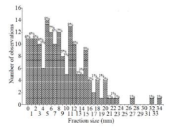
Fig. 5. Distribution of length of feedstock material fraction
