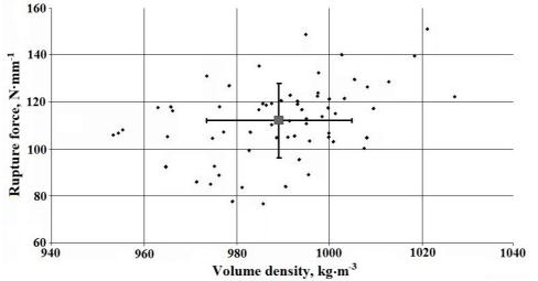
Fig. 6. Relation between rupture force and volume density of produced briquette samples
